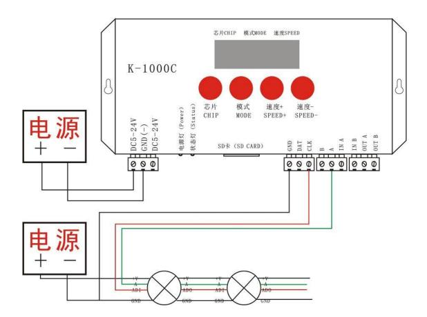
1. Like the above diagram, wired the line and start the controller, press "CHIP" and "MODE" at the same time switch to coding mode, adjust to Chip: 61 that is UCS512A or B coding mode, as below:
