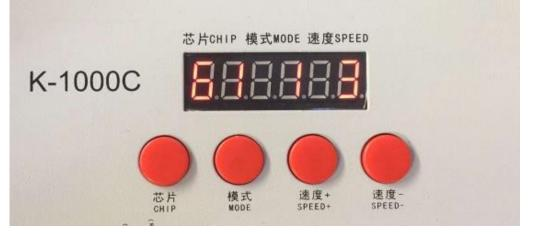
NOTE:61 means UCS512A or B coding mode; 62 means WS2821 coding mode; 63 means SM DMX512AP; 64 means UCS512-C; Ch.: 03 means the coding channel is 3 channels
