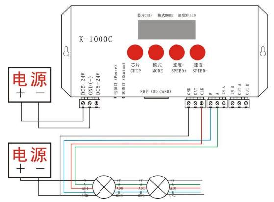
Single signal wiring diagram:
